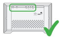
Regularly check the LED light indicators on the Network Termination Device. If they are not showing a green light, refer to the guide on page 9.
