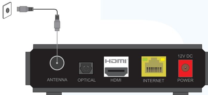
1. Plug one end of the existing antenna cable into the antenna wall socket, or leave if already connected to the wall.
