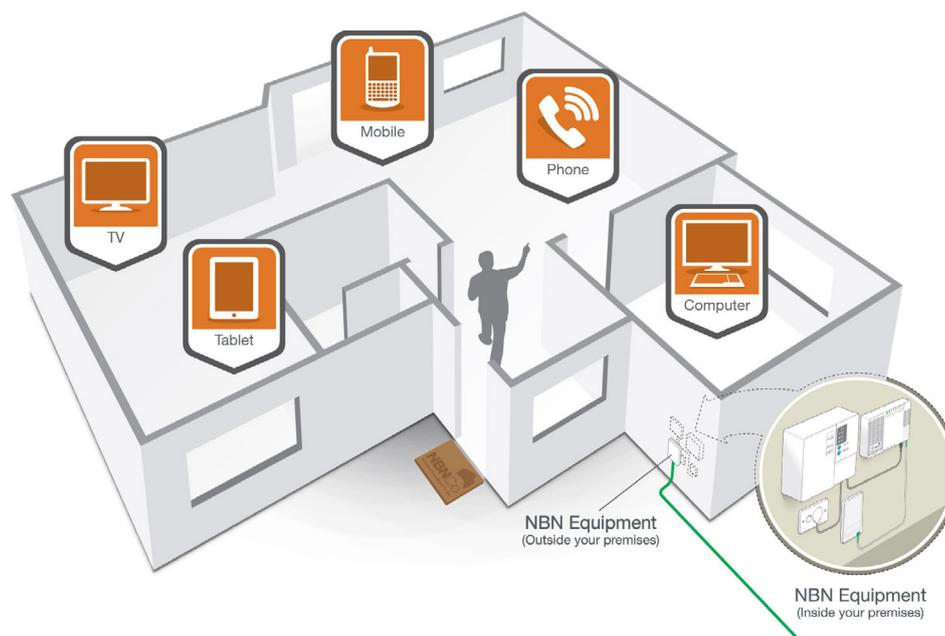
Customer telephone and data cables cannot extend outside or between buildings. They are susceptible to lightning and are a potential hazard as the lightning can be transferred between different ports of the Network Termination Device to any equipment they have connected.
